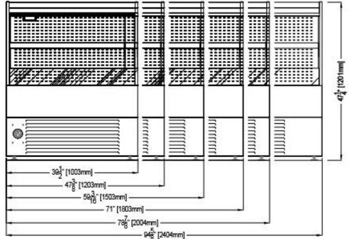
**STANDARD: MURO H13-1 A90SQ FRONT ELEVATION (CUSTOMER SIDE)**
