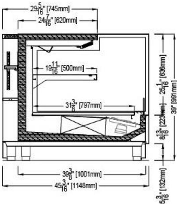
**MURO H13-2: REMOTE CONDENSING UNIT W/ BACK SHELVING**
